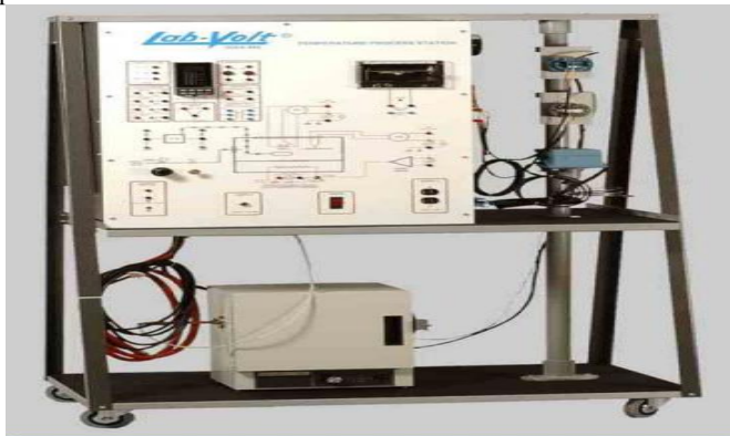
Fig. 1: LAB-VOLT - temperature process station Model 3504.
