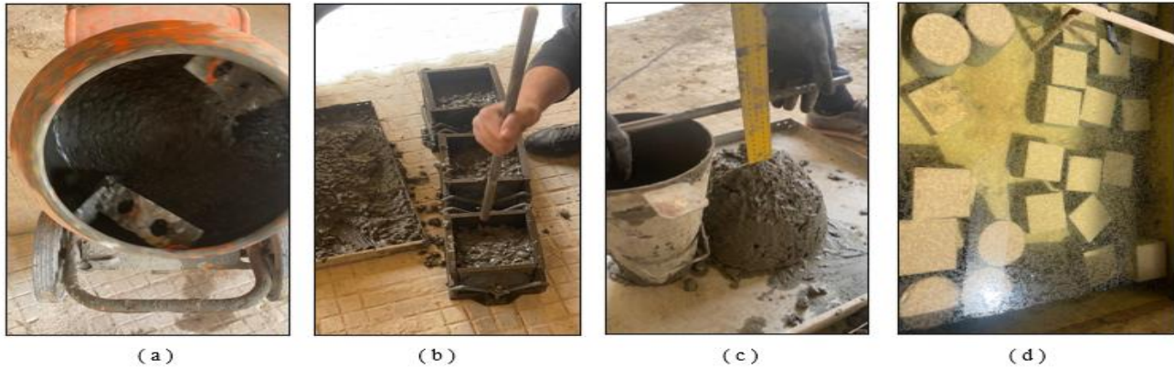
Fig. 5: Specimens preparation stage: (a) Mixing, (b) Cast and compaction, (c) Slump test, (d) Curing
