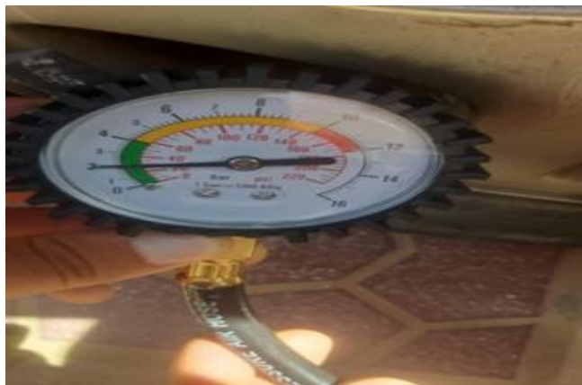
Fig. 6: Measurement of tire pressure (bar) using a gauge.
