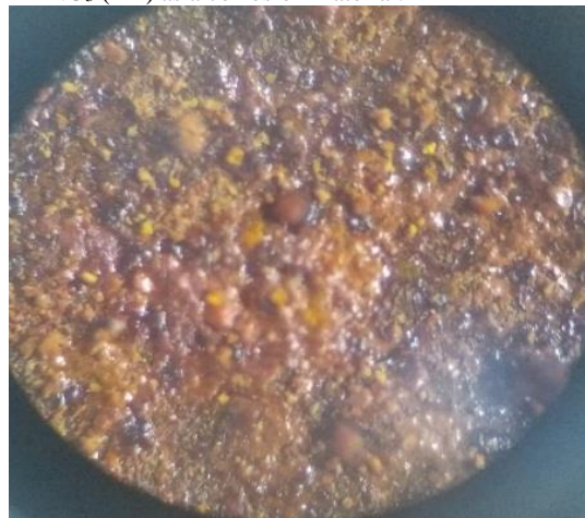
Fig. (22): Show, the corrosion of Fe by HNO 3 (1M) without mango inhibitor.
