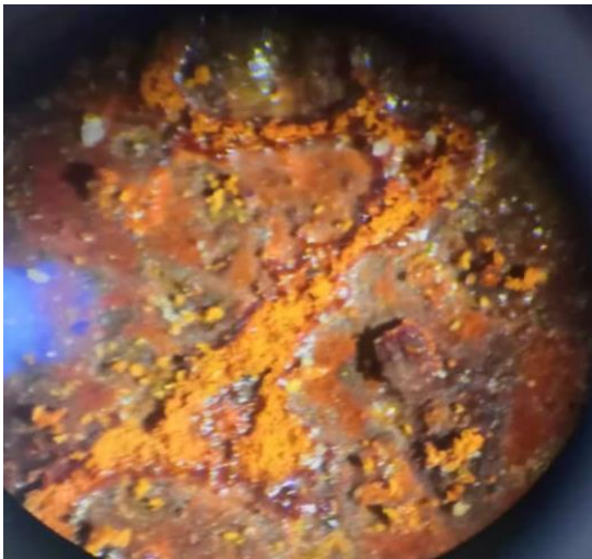
Fig. (25): Show Fe after corrosion by HNO 3 (1M) without berry inhibitor.
