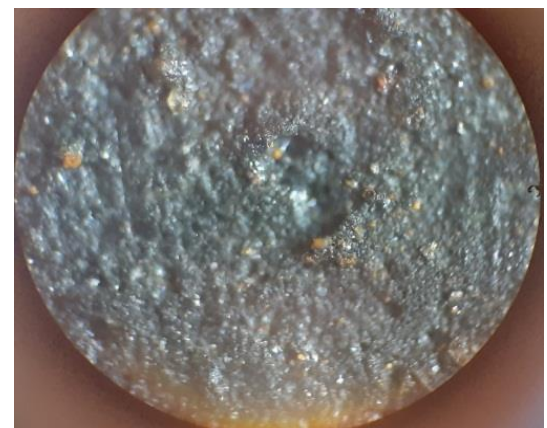
Fig. (17): Show, the corrosion Fe alloy of oil pipeline r by 1M HNO 3 without any berry inhibitor.
