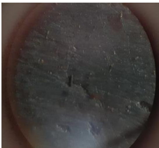
Fig. (29): Show Fe after corrosion by HCl (1M) with mango inhibitor.
