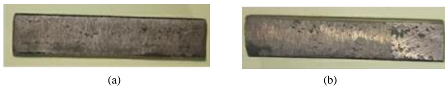
Figure 4: (a&b)photo of specimen immersed in water with inhibitor
