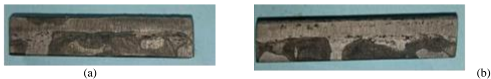
Figure 5: (a & b) photo of specimen immersed in water without inhibitor
