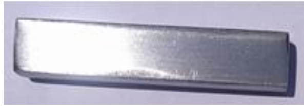
Figure 3: photo of specimen before the immersion
