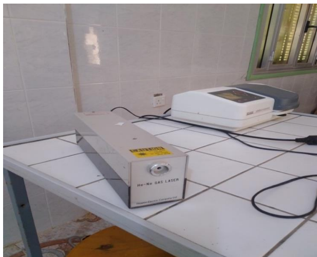
Fig.1. He – Ne gas laser device and JENWAY 6300 spectrophotometer
