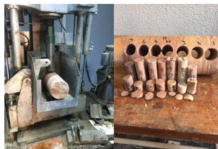
Figure 2. Process of cut core sample & shape of cores after cut process.
